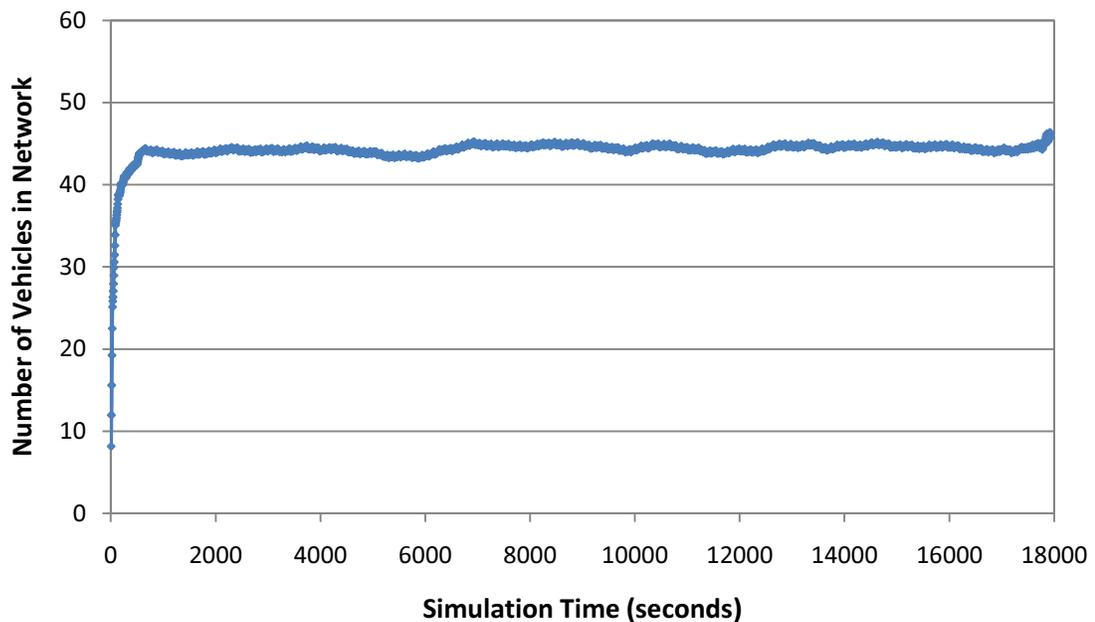
**Figure 2. Welch's Method for 5<sup>th</sup> Street Model, window size 100, five hour run**
