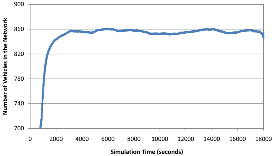
**Figure 41. Welch's Method for large network, 50 replications,  $w = 150$**
