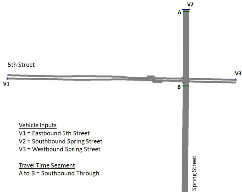
**Figure 7. Location of Performance Measures for Single Intersection Model**
