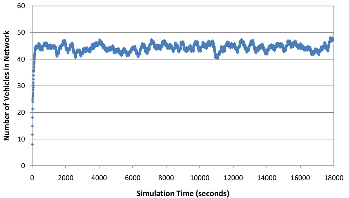
**Figure 14. Welch's Method for 10 Replications and window size 20**
