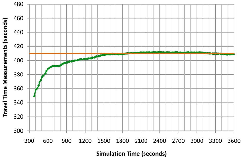
**Figure 27. Welch's Method for Travel Times, large model, 40 replications,  $w = 50$**
