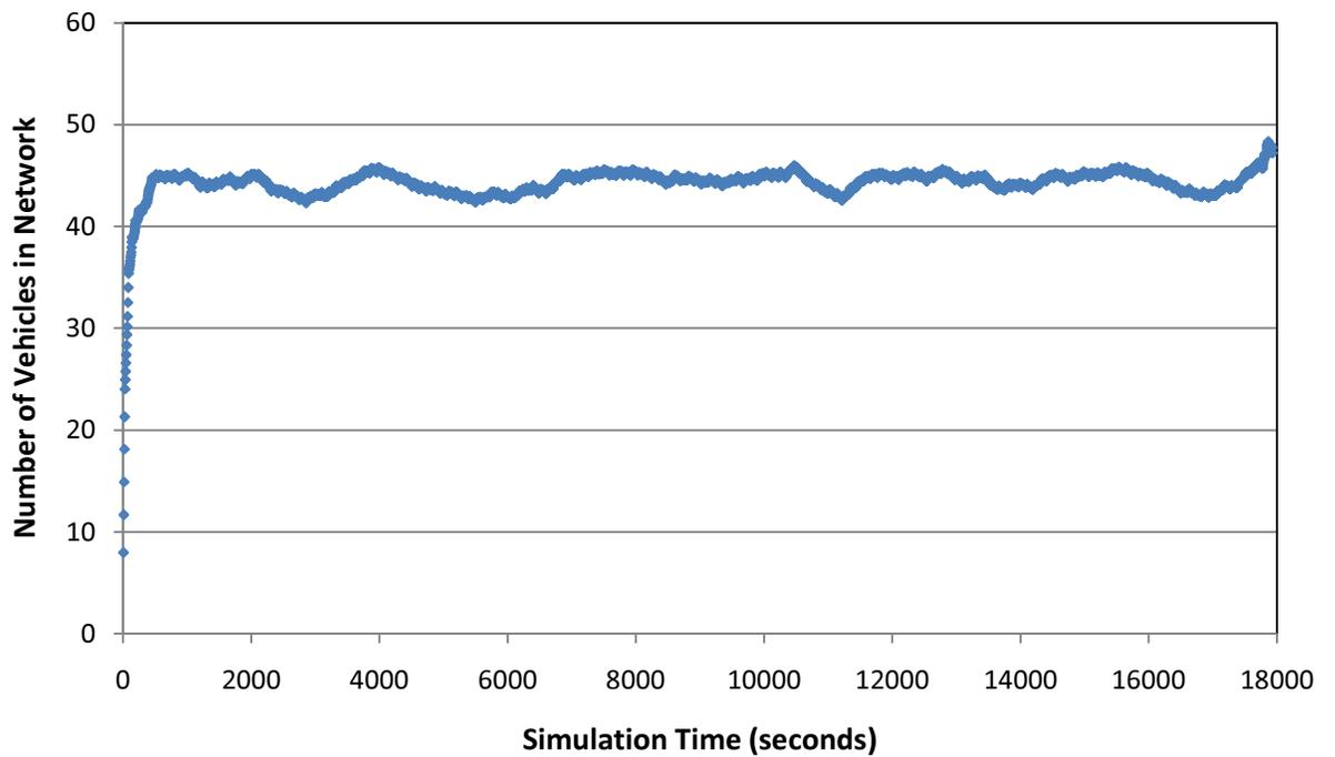
**Figure 18. Welch's Method for 10 Replications and window size 75**
