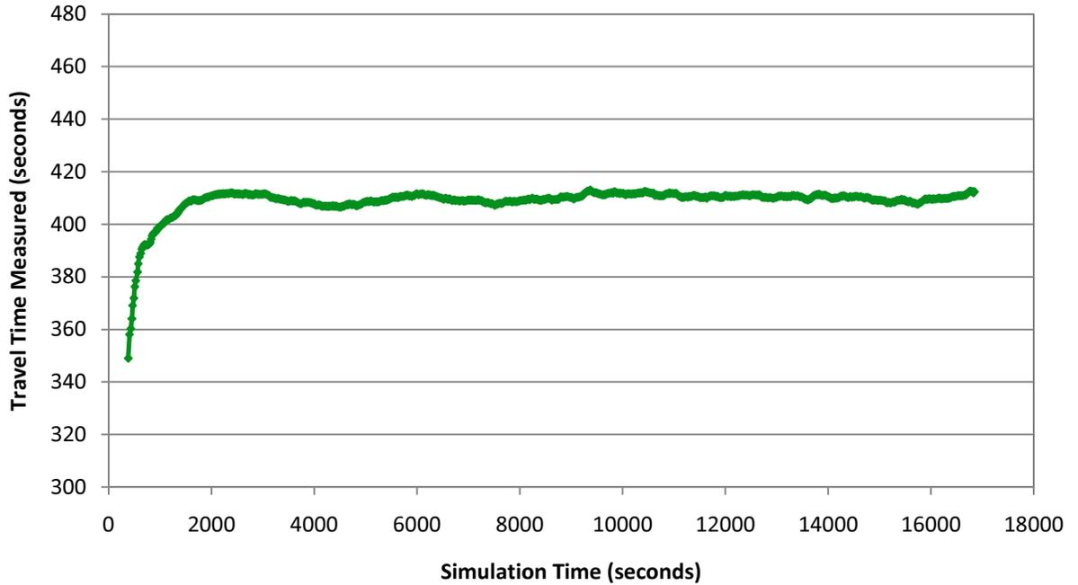
**Figure 26. Welch's Method for Travel Time, large model, 40 replications,  $w = 50$**
