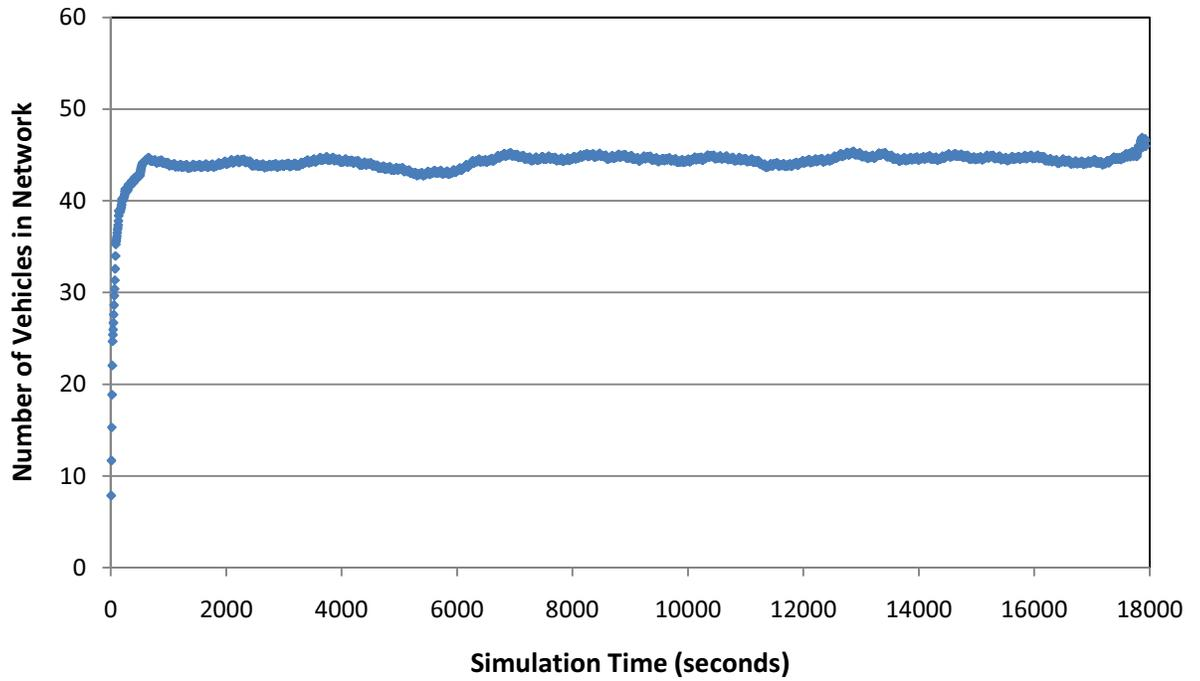
**Figure 21. Welch's Method for 30 Replications and window size 100**
