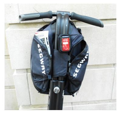
Figure 32. GPS recorder Instrumented on Segway
