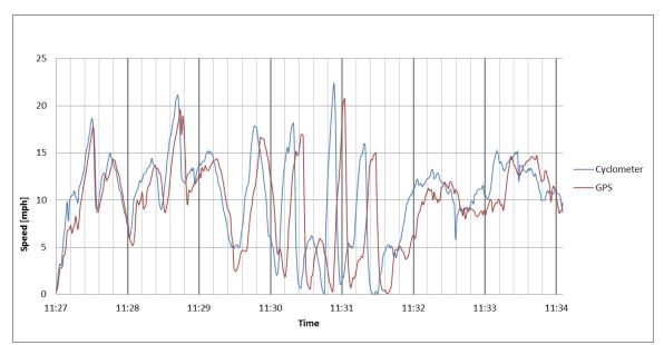
Figure 21. Example of Cyclometer Speed with Clock Error
