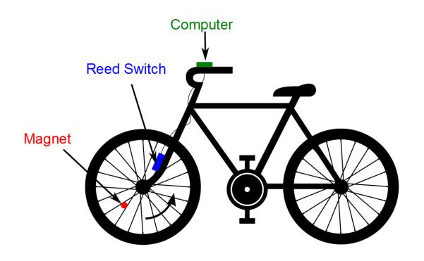
Figure 18. Diagram of Cyclometer Installed on a Bicycle (Credit: Lance Ballard)
