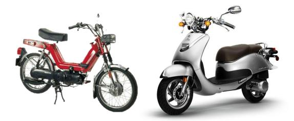
Figure 4. Examples of a Moped (left) and a Motor Scooter (right) (Lance Powersports, 2012; MRA, 2012)
