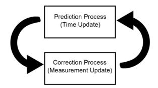
Figure 15. The Kalman Filter Cycle
