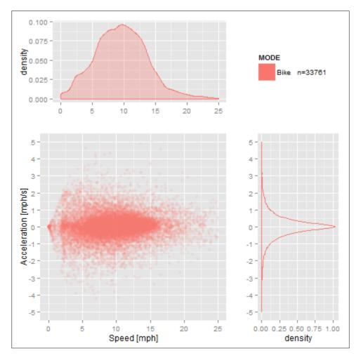
Figure 38. Bicycle Speed and Acceleration
