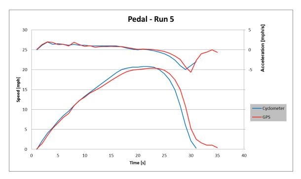
Figure 26. Lab Test – Pedal Speed – Run 5
