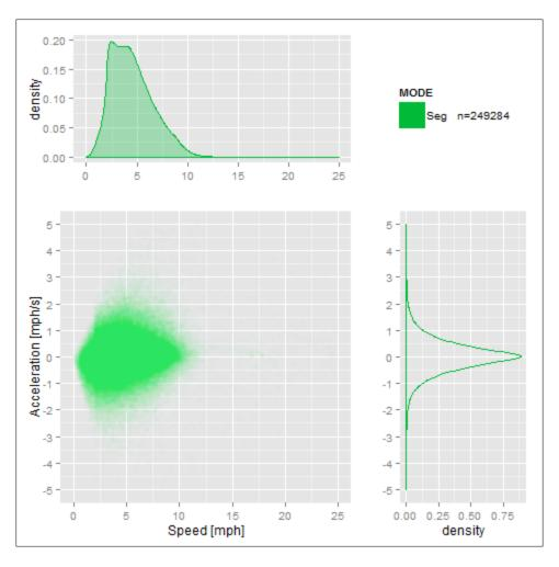
Figure 37. Segway Speed and Acceleration
