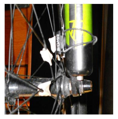
Figure 20. Magnets and Cyclometer Reed Switch Installation
