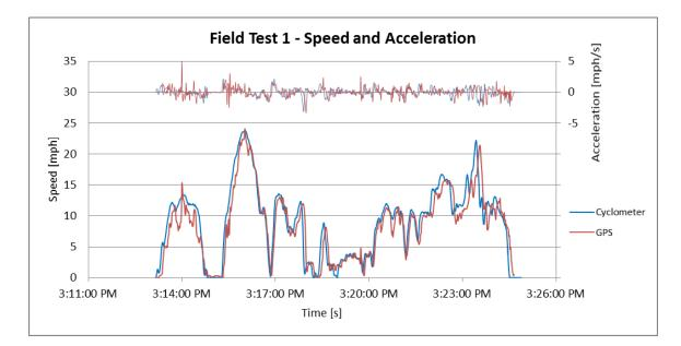
Figure 28. Data Collection Method Validation Field Test 1 Speed and Acceleration
