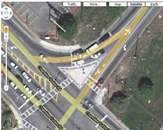
**Figure 46: Ramp Turn Lanes at the Northeast Approach**
